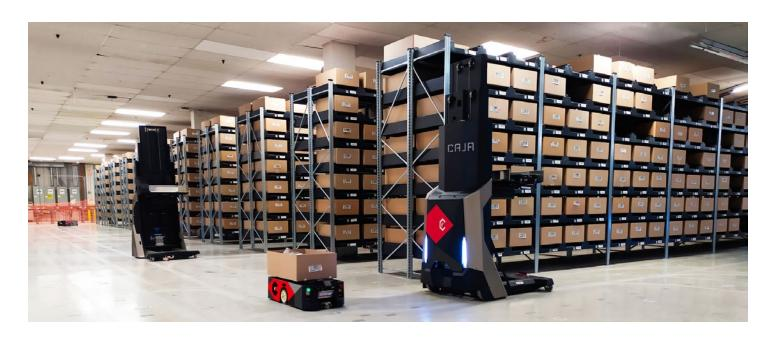
adding robots and storage only when needed. Their relatively short deployment time (6 months or less) allows for a quick transition to a micro-fulfillment strategy.
